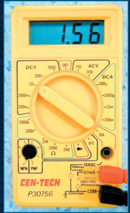
12. Reading a AA battery while in the 20 DCV scale.
